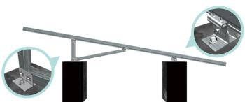
2. Fasten the T Jointer on the front of GT5 Pre-Assembled Supports to the T Anchor Plates; and fasten the Back Supports and the Inclined Support to the Corrugated T Anchor Plate
